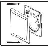
**9.** Align tabs on snap-fit grille with slots in baffle, gently press grille into place.
